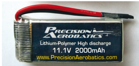
The power source is the 2000 mAh three cell Lipo pack.
